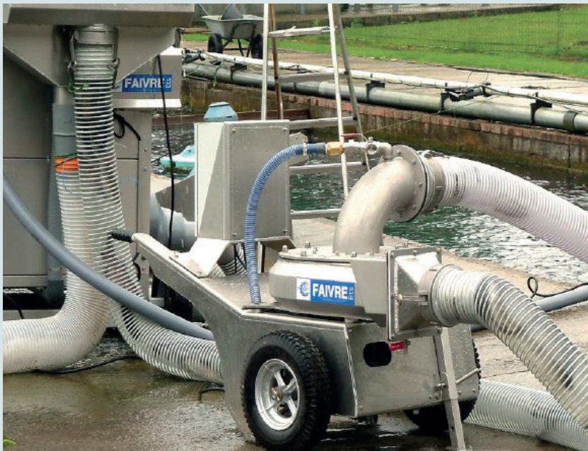
Optimum choice of materials. Alu frame and AISI 316 pump housing.
