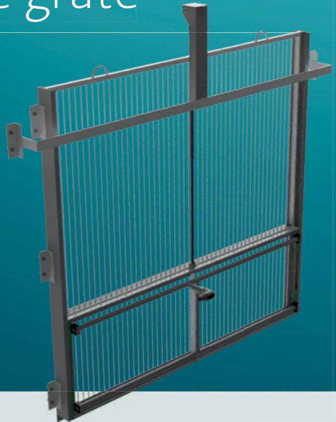
The grate includes several functions that must be adapted to the water flow, fish sizes, tank dimensions, etc. The weight and external dimensions will vary according to size/capacities. The main drainage grate is preferably mounted on a concrete structure and preferably in front of the drum filter in the drainage tank for waste-water treatment. It consists of a grate with an actuator-controlled flushing and brushing system for efficient washing/cleaning.
